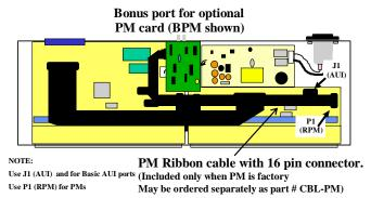
**NOTE:** The PM will still function if connected to header J1/B of the circuit board corresponding to ports 1-12. However, this is not advised, as the port will not be recognized by an SNMP Agent (if one is present).
